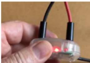
► If the receiver is correctly connected, the battery automatically charges.
