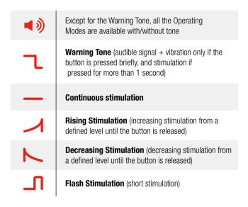
To change the operating mode, keep the program button (9) pressed. The LCD screen then displays in sequence the different symbols.
